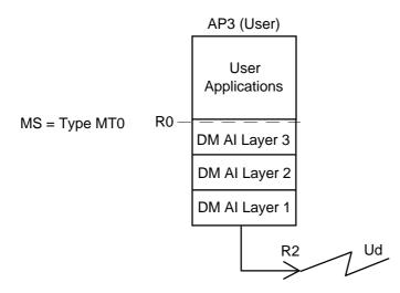
Figure 8: MT0 protocol stack for DM air interface
