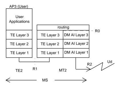
Figure 9: MT2 protocol stack for DM air interface
